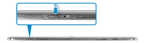
**Power button LED** is lit while the computer is turned on.
